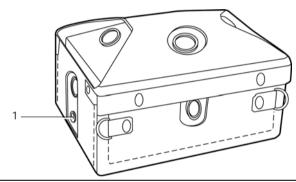
The charge connector is located on the side of the multi-transmitter.
