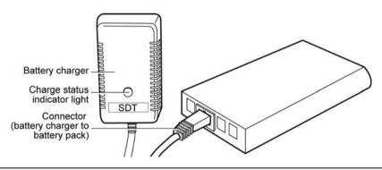
Connection of the battery charger onto the battery pack.
