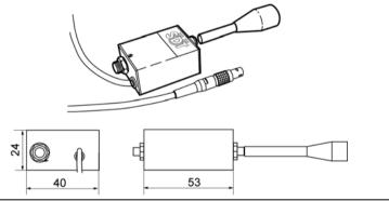
External view of the mass air flow sensor.
