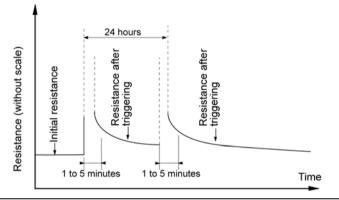
Automatic reset curve of the chemical fuse.
