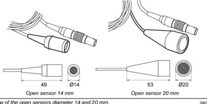
View of the open sensors diameter 14 and 20 mm.
