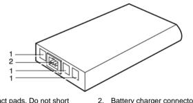
1. Battery contact pads. Do not short 2. Battery charger connector. circuit.
