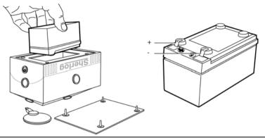
The battery is accessible from the bottom and the obligatory arrangement of the battery. 104
