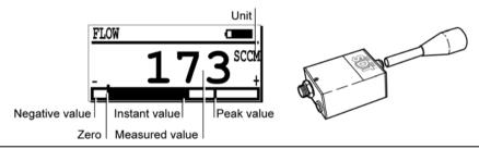
The Sensor options menu with mass air flow sensor.
