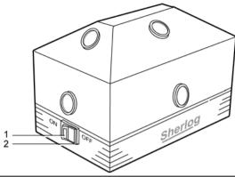
The on-off switch (1) and battery control indicator (2).
