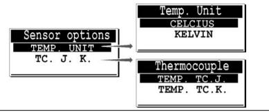
The Sensor options menu with thermocouple interface.
