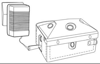
Recharging a battery without removing it.
