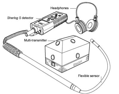
The complete testing equipment: detector, flexible sensor, multi-transmitter, headphones. 266
