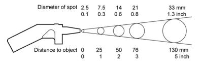
The spot size increases with distance from the probe tip, as shown.
