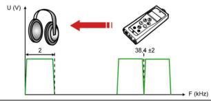
The main function of the Sherlog S is converting high frequency signals into audible.
