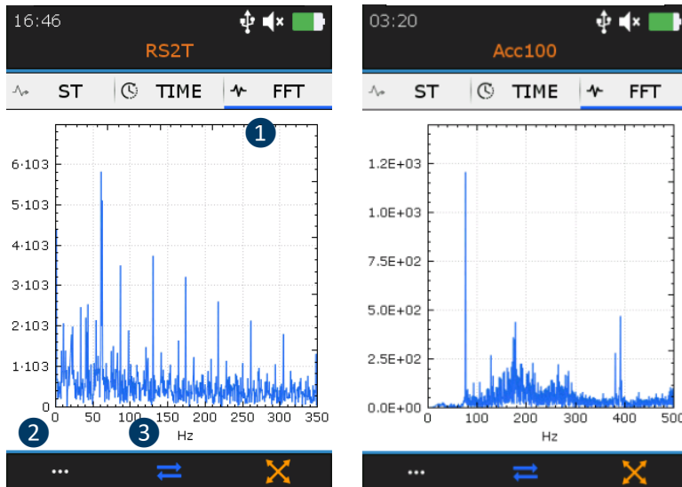
Figure 15-1: Spectrum view ultrasound right and vibration left
